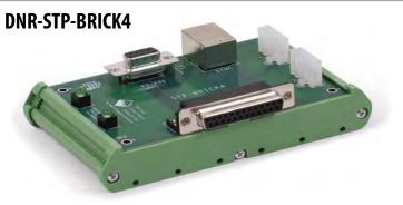
The optional DNR-STP-BRICK4 (shown above) provides easy connections to the 25-pin D-Sub diagnostic/power/sync connector. Power (for non POE or backup) connections are provided via standard UEI power supply Molex connectors. RS-232 connections are through a 9-pin D-Sub connector while sync connections are provided via a RJ-50 connector. Please see the accessories section below for order info.
