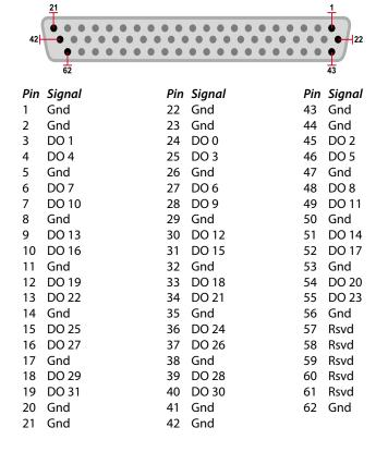
**Note:** For rated performance all ground pins should be connected to the external ground.
