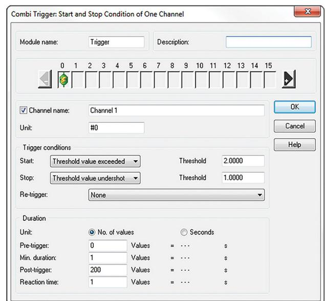
A variety of trigger modules are available to control the data flow in the worksheet. The Combi Trigger module dialog box is shown here
