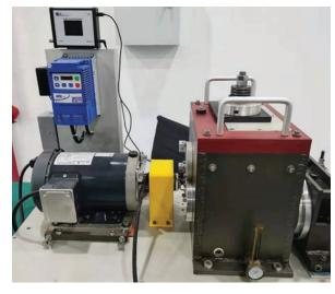
The test bench simulates multiple operating conditions, providing valuable feedback to the operator. Load analysis data gives engineers the ability to detect bearing and gear fault situations.
